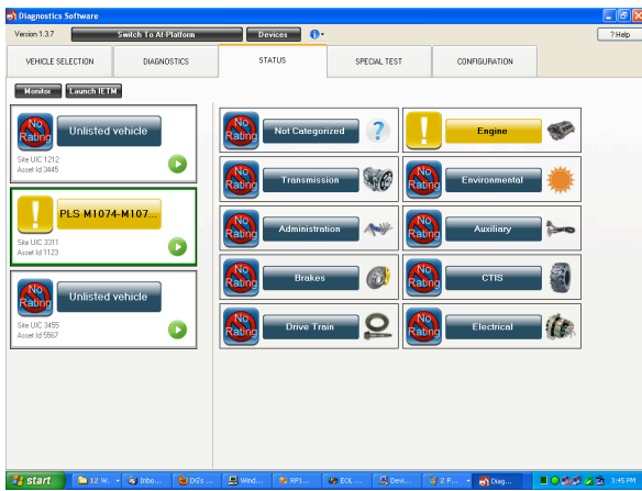
Figure 10: DS Displaying Vehicle Health Status, Courtesy DG Technologies
